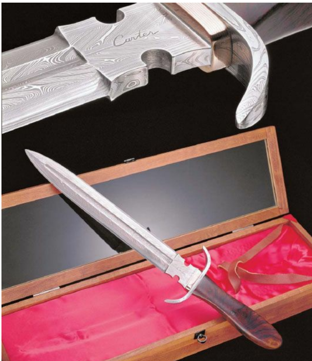
Nine-inch custom dagger in 5-bar composite damascus steel with fuller, Damascus guard and mokume hardware. All work by author, including presentation case.
