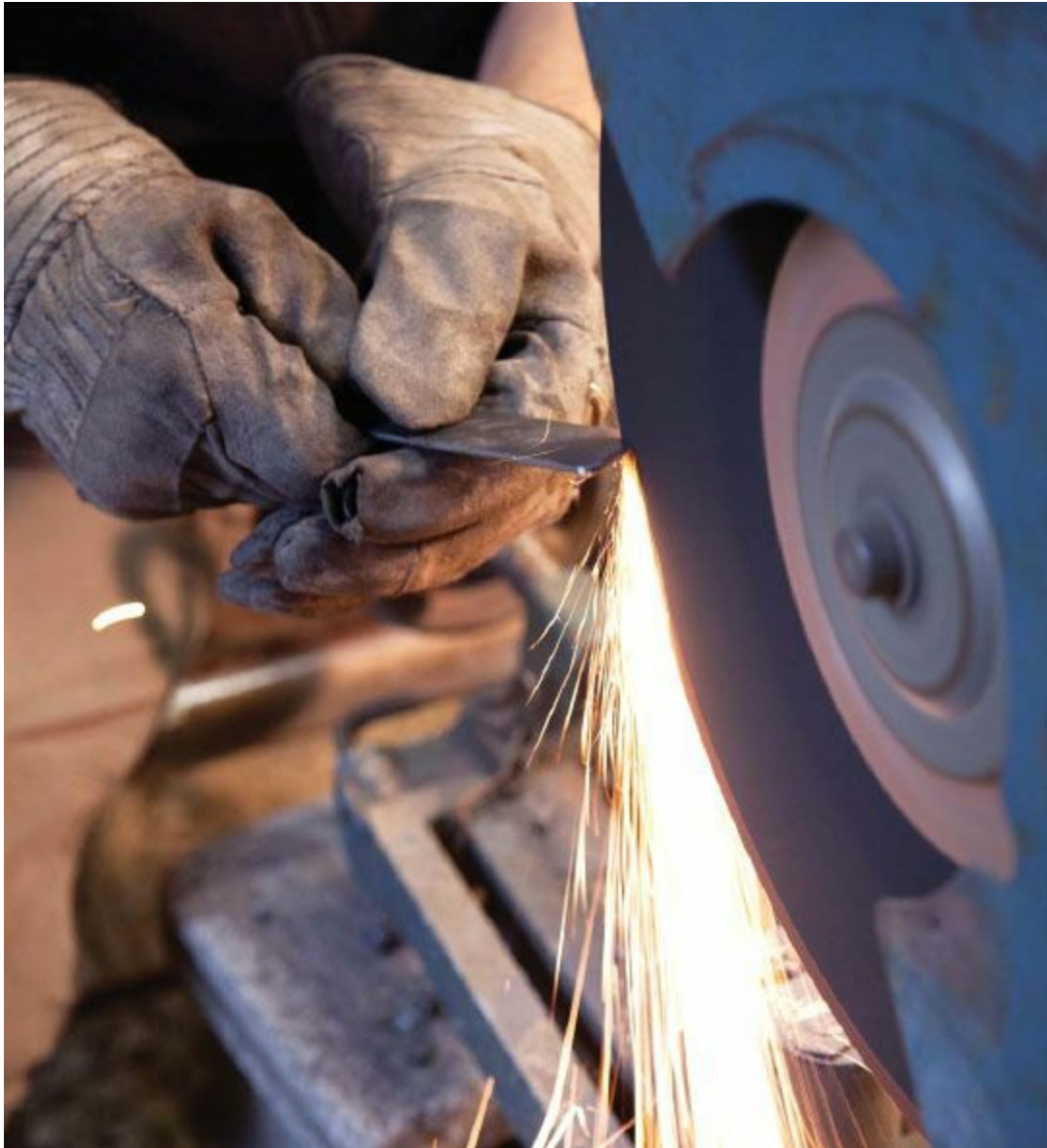
Cutting out patterns with the circular chop saw. Notice the safety gear.
