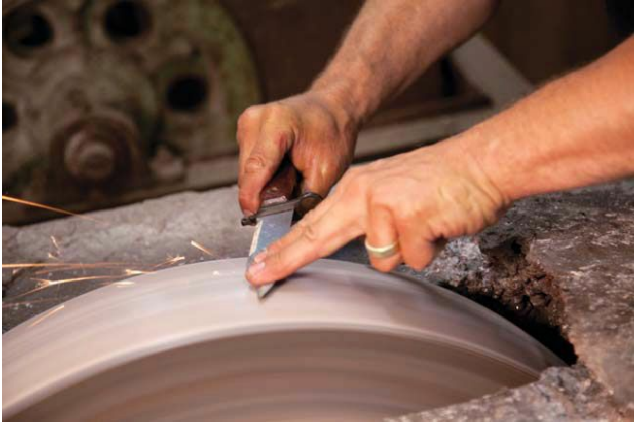
Author regrinds a Russian AK-47 bayonet on the Japanese rotating water stone sharpener.
