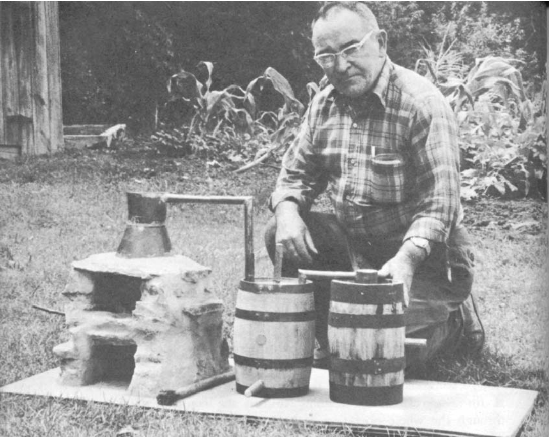
PLATE 262 Buck Carver kneels behind a one-gallon still he made for the Foxfire museum. The still is authentic in every detail from the flue of the furnace to the tin-locked copper joints in the cooker and condenser to the chestnut barrels Bill Lamb made for the model.
