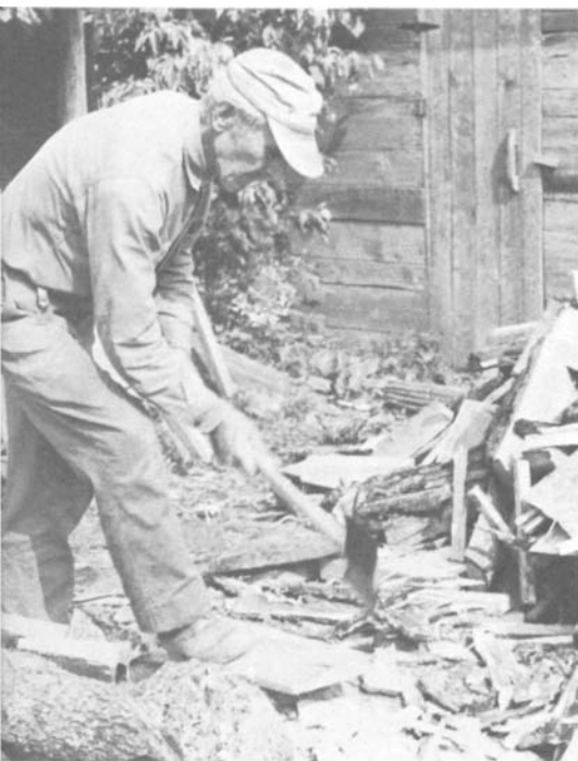
PLATE 27 . . . "barks" it, or removes the bark and outer layers of fiber.
