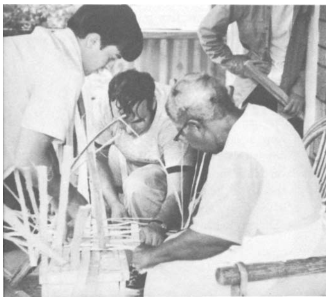
PLATE 159 The hamper requires twenty-four heavy ribs, each about an inch wide. Crease each rib, while green, in two places, thus dividing it into three sections, each twenty-two inches long. Here Beulah creases one rib. All knots and rough places should be hammered out so they will not interfere with the weaving.
