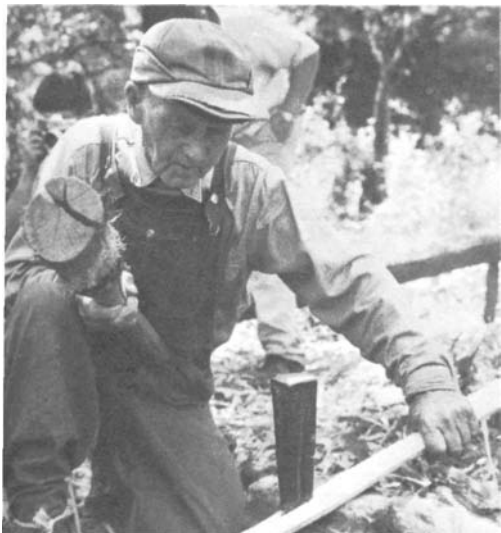
PLATE 153 Now each quarter is halved thus converting the original trunk into eighths. Lon prefers using the steel wedge in this phase as its edge is sharper than that of the glut.
