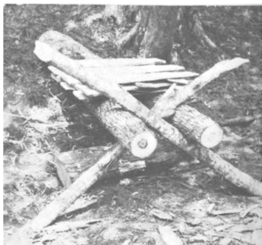
PLATE 28 The bolt now goes to the board "brake" to be converted into shingles. The brake, in this case, is the narrow "Y" crotch of a black gum tree cut about six feet long. The single end is propped up, and two stout poles are crossed in the double end. No nails or other braces are needed, for these poles wedge firmly enough to hold the end up. As one man said, "They work contrary to each other."
