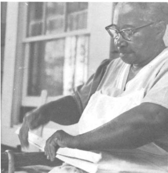
PLATE 159 The hamper requires twenty-four heavy ribs, each about an inch wide. Crease each rib, while green, in two places, thus dividing it into three sections, each twenty-two inches long. Here Beulah creases one rib. All knots and rough places should be hammered out so they will not interfere with the weaving.
