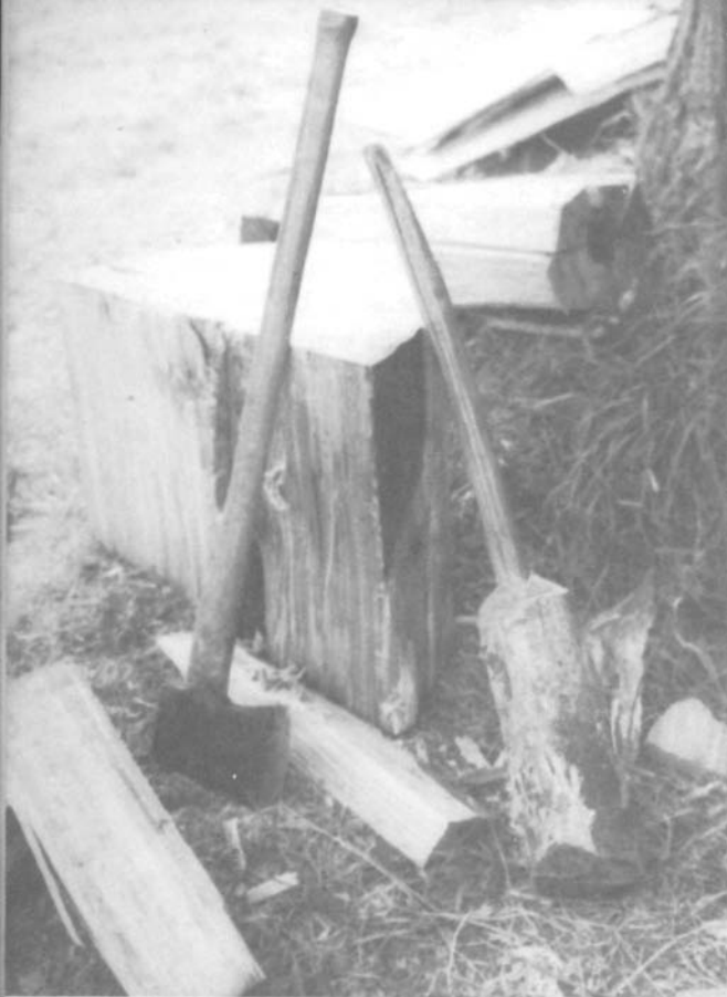
PLATE 10 A poleaxe and a maul leaning against a two-foot section of oak that is being split into shingles or "boards."
