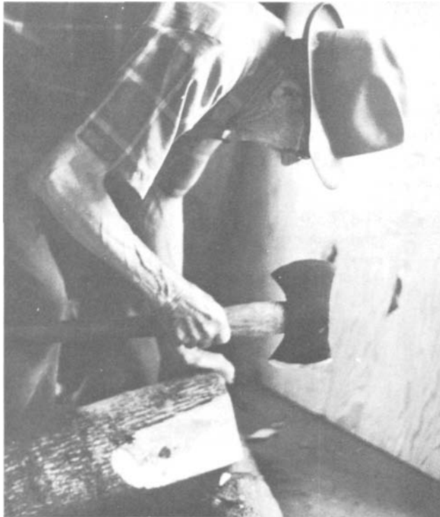
PLATE 62 With an axe, hew the two sides of the log back twelve inches from the end.
