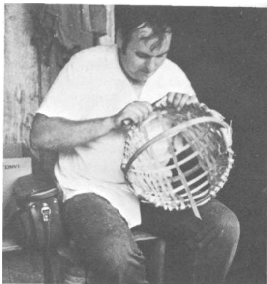
PLATE 178 Here, the basket is well over half completed. All the ribs have been worked in.
