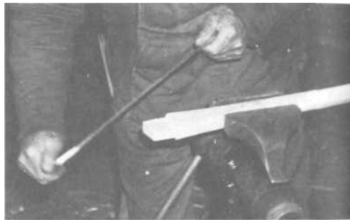
PLATES 85-89 The bases of the twelve spokes are now shaped, as shown in PLATES 85-89. These are the "tenons" that fit the twelve slots, or "mortises," cut in the hub. First the draw knife cuts across the grain to the desired depth (Plate 85); then the knife is held parallel to the grain of the wood and struck with an axe or hammer (Plate 86). The back of the spoke is then sloped to work against the slope of the mortise (Plate 87), and the edges tapered so the tenon will slip easily into the mortise (Plate 88).
