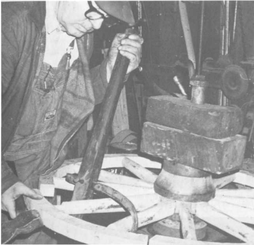
PLATES 101-102 When the spokes are ready, the felloes are laid, section by section, on the ends of the spokes, and marked on their inside curves so holes for the ends of the spokes can be drilled in the proper places. Once drilled, the felloes are mounted in place. John calls the tool he is using a "spoke puller." It pulls the spokes closer together so they can fit the holes in the inside of the felloes. As the felloe is driven on ( Plate 102 ), the spokes spread back apart into their natural positions.
