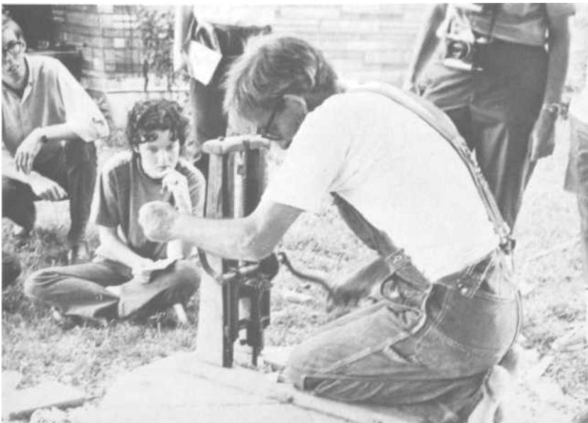
PLATE 138 He now begins work on the buckets themselves. Nine holes are drilled in each bucket as shown.
