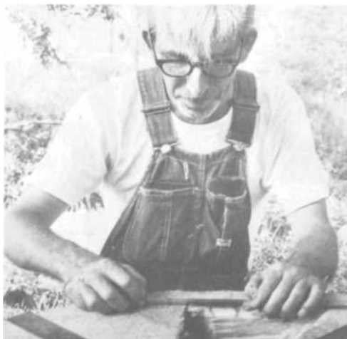
PLATE 142 As he progresses, he continually checks and rechecks his measurements to make sure he is shaping the sides of the bucket correctly.
