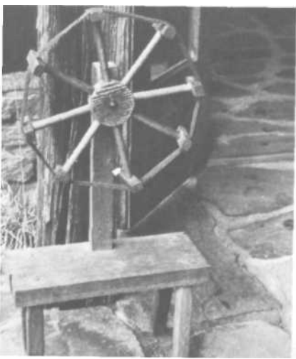
PLATE 240 Shown here is one type of reeler that is relatively easy to make. It can be put together either with nails or with wooden pegs. One-inch holes are drilled through the bench at a slant, and the ends of the legs are tapered to the holes with a drawknife. Almost any type of wood is suitable.
