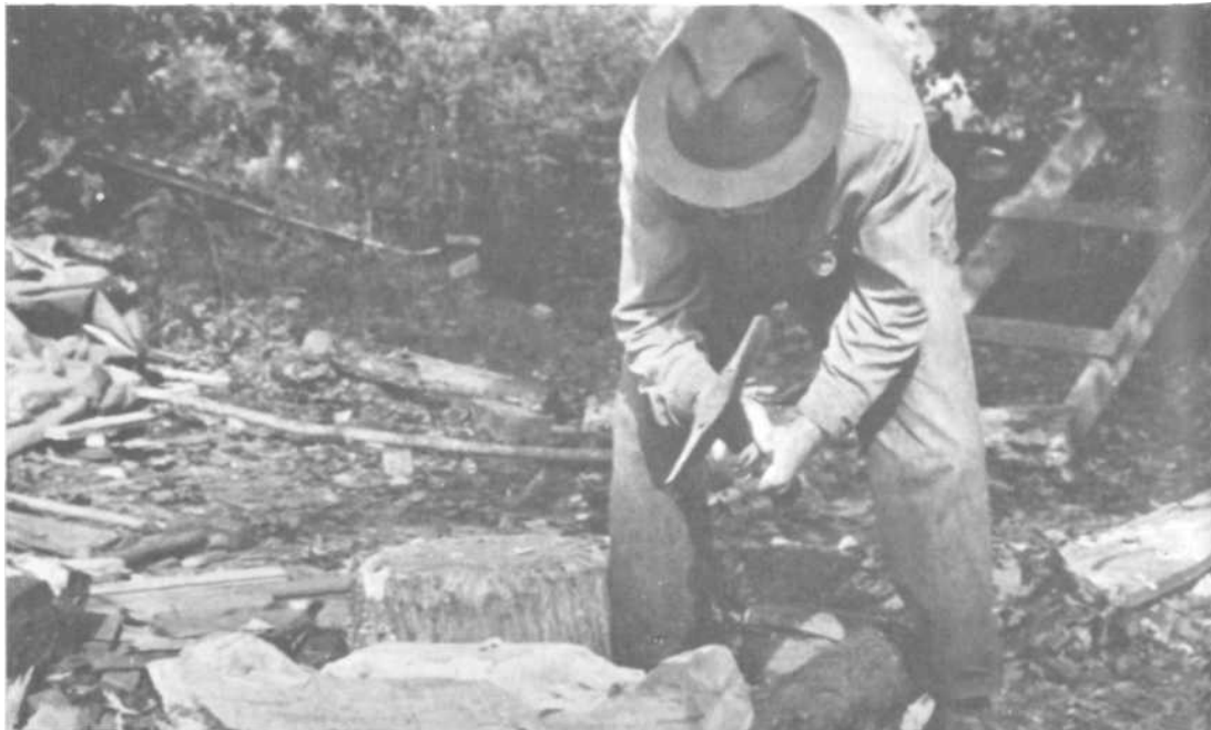
PLATE 66 Next, with an axe or hatchet, and turning the yoke from side to side as necessary, the yoke is hewn out in rough form. A drawing knife is used for the final smoothing and shaping.
