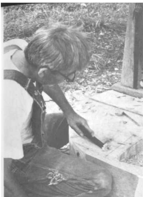
PLATE 143 In the second bucket, Sam finds a piece of wire sticking out of the middle of the wood. Here he tries to ease it out without dulling the edge of his chisel.
