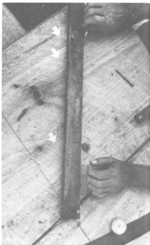
PLATE 134 Sam now finds dead center of the top surface. He drives a nail through a stick of scrap wood into dead center, measures out eighteen inches from dead center on the stick, and drives a second nail through this point. With the point of the second nail, he scribes a circle thirty-six inches in diameter on the top surface.
