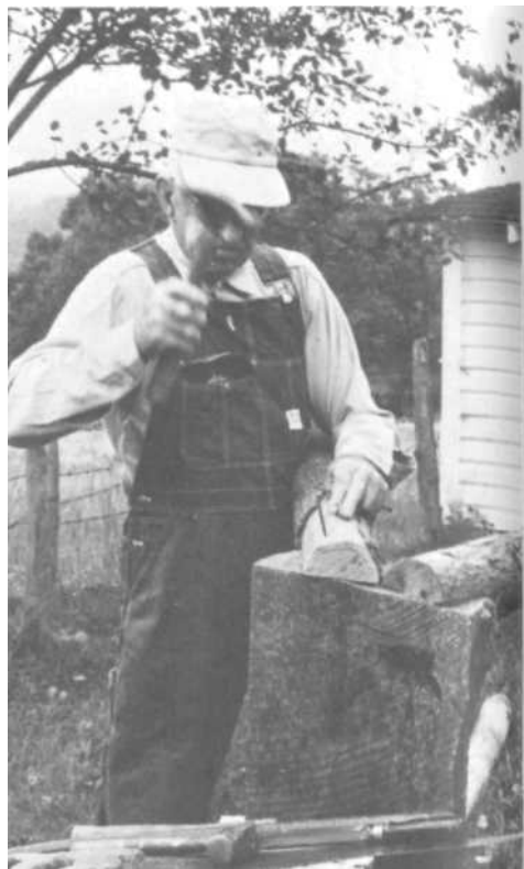
PLATES 320-322 Mr. Dickerson notches the ends of the three legs to fit the battling bench, and then nails them into place. The bench has three legs so that it will set steady, even on rough ground.
