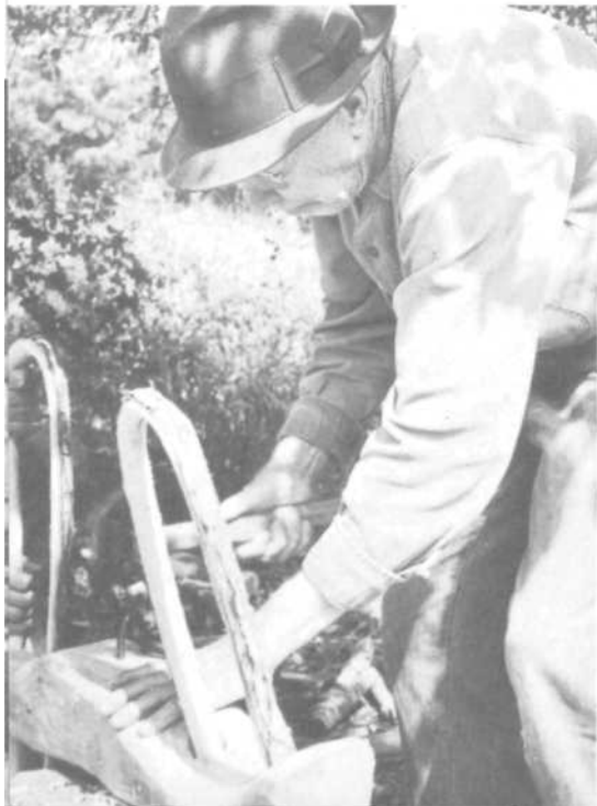
PLATE 73 . . . and then got out the steeple and nailed it into place in the bottom center of the yoke. Chains used to pull wagons and sleds are hooked to the steeple's ring. The weight of the load behind pulling on the ring holds the yoke firmly in place on the oxen's shoulders.
