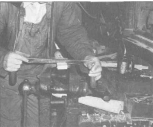
PLATES 85-89 The bases of the twelve spokes are now shaped, as shown in PLATES 85-89. These are the "tenons" that fit the twelve slots, or "mortises," cut in the hub. First the draw knife cuts across the grain to the desired depth (Plate 85); then the knife is held parallel to the grain of the wood and struck with an axe or hammer (Plate 86). The back of the spoke is then sloped to work against the slope of the mortise (Plate 87), and the edges tapered so the tenon will slip easily into the mortise (Plate 88).
