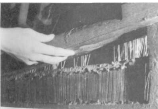
PLATE 258 Beater raised to show groove cut to hold reed.
