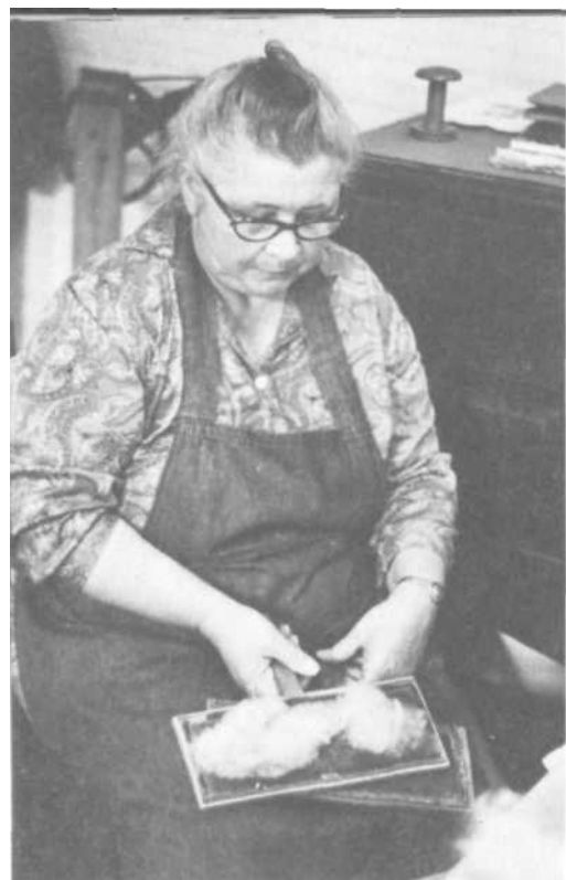
PLATES 205-207 In making rolls for spinning, Margaret uses a set of fine-toothed "roll cards." She takes one bat, pulls it apart, distributes it over the top card (Plate 205) as before, and combs the wool several times (Plates 206—207) as before (motions A and C).
