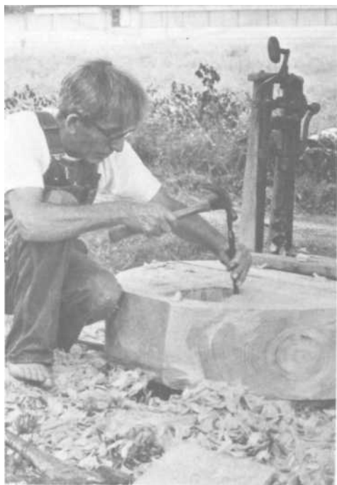
PLATE 142 As he progresses, he continually checks and rechecks his measurements to make sure he is shaping the sides of the bucket correctly.
