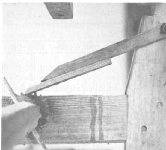
PLATE 289 Brace (clutch) mounted to side (inside) of frame to articulate with cogs and hold cloth beam steady and in place so threads are kept taut.
