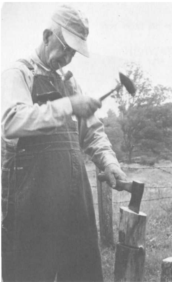
PLATES 320-322 Mr. Dickerson notches the ends of the three legs to fit the battling bench, and then nails them into place. The bench has three legs so that it will set steady, even on rough ground.
