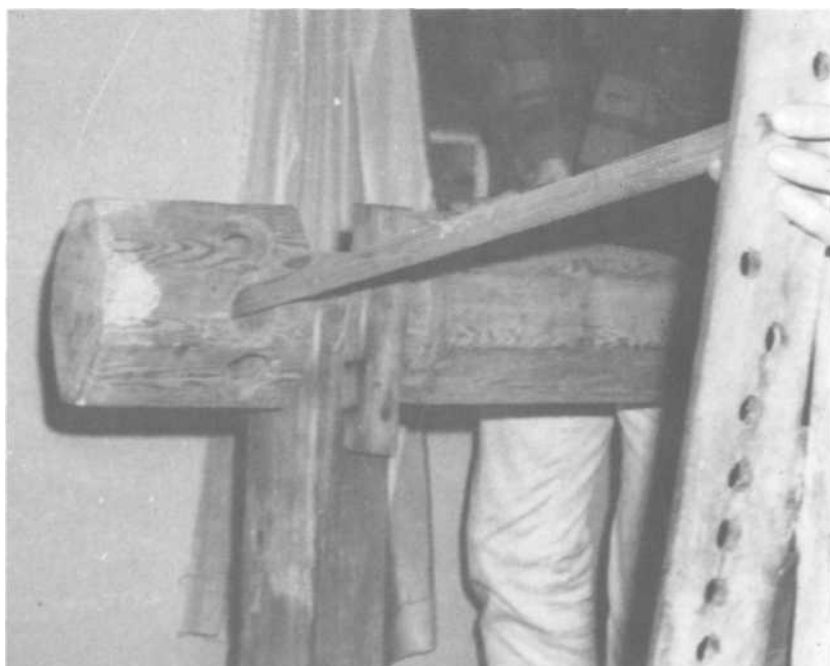
PLATE 272 A stick runs from any of the holes in the end of the beam to any of the holes in the slat shown (see also Plate 286 ). This keeps the warp taut while weaving.
