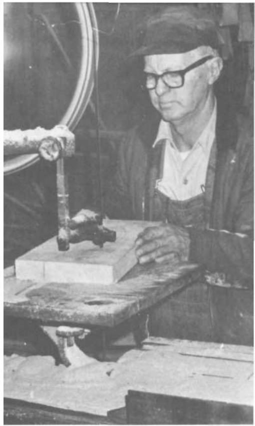
PLATE 94 Instead of using the fellow saw, John now uses a band saw to cut out the felloes.
