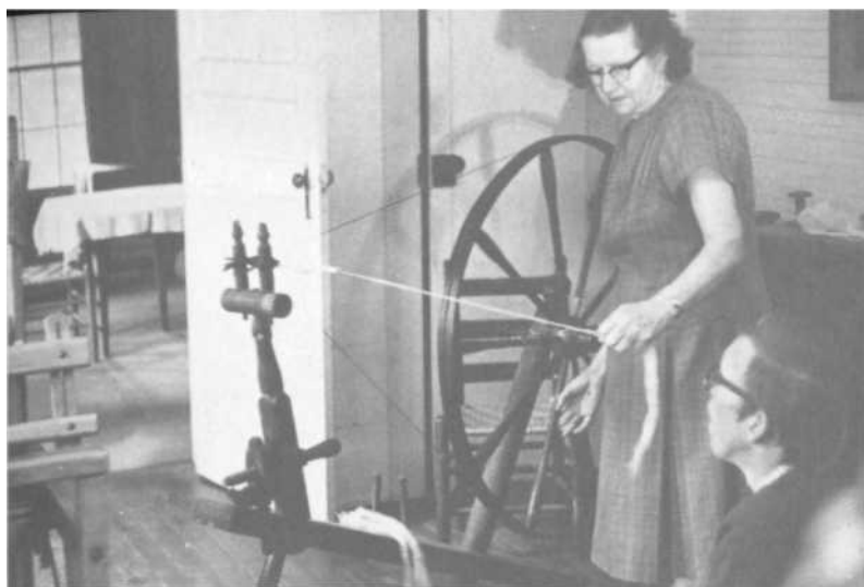
PLATE 218 Keeping the wheel turning, she draws the thread back until it is about three feet long.
