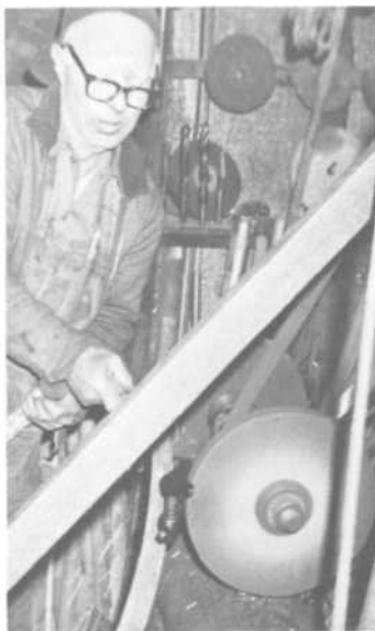
PLATES 107-109 The tire that John had planned to use on our wheel was too large, so he cut out a section ( Plate 107 ), rewelded it carefully back together on top and bottom ( Plate 108 ), and ground off the rough edges ( Plate 109 ).
