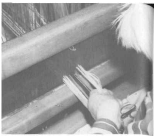
PLATE 304 Make sure the threads are tied on with an equal amount of tension.
