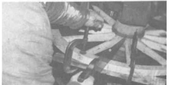
PLATE 103 When the felloes are in place, John takes a hand saw and saws down between each seam to insure that they meet flush, and are lined up correctly.
