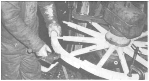
PLATES 101-102 When the spokes are ready, the felloes are laid, section by section, on the ends of the spokes, and marked on their inside curves so holes for the ends of the spokes can be drilled in the proper places. Once drilled, the felloes are mounted in place. John calls the tool he is using a "spoke puller." It pulls the spokes closer together so they can fit the holes in the inside of the felloes. As the felloe is driven on ( Plate 102 ), the spokes spread back apart into their natural positions.
