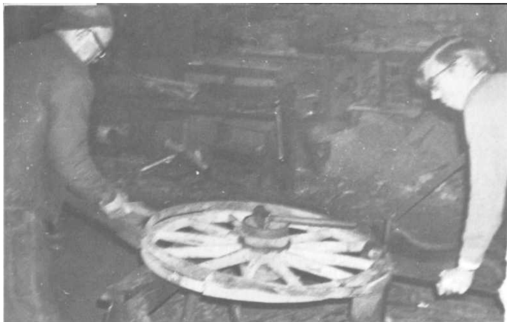
PLATES 111—113 Moving quickly, he carries the tire to the wheel, has a second person clamp down on the opposite side to keep the tire from flipping up (Plate HI), and pulls the tire over the rim of the wheel with a "tire puller" (Plates 112-113).
