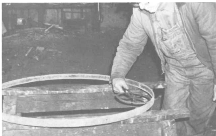
PLATES 105-106 With a traveler, John checks the circumference of both the wheel and the metal "tire" to make sure the fit is good. The tire should be about a half-inch smaller in inside circumference than the outside circumference of the wheel itself. This insures a tight fit.
