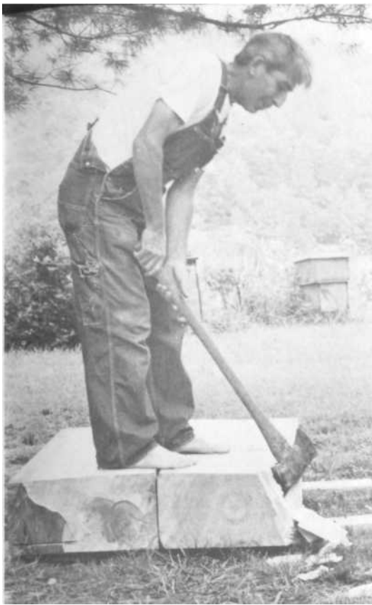
PLATE 137 With an axe, he hews the wheel out round.
