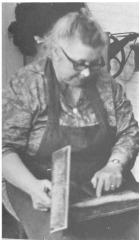
' LATE 209 Then, using several strokes of motion E, she gently nudges the roll backwards. This helps to gather the fibers and consolidate the wool into an actual «oll." When the roll is at the back of the bottom card
