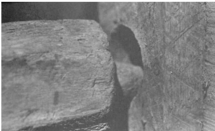
PLATE 282 This end of cloth beam is hewn into a knob to fit into hole in loom frame.
