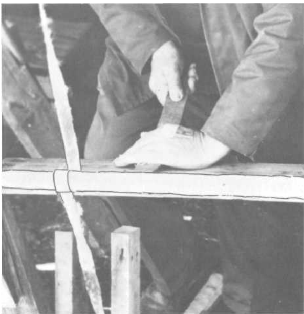
PLATE 176 Each time the pedal is depressed, the pole pulls the pedal back to the return position, spinning the stock in the opposite direction.
