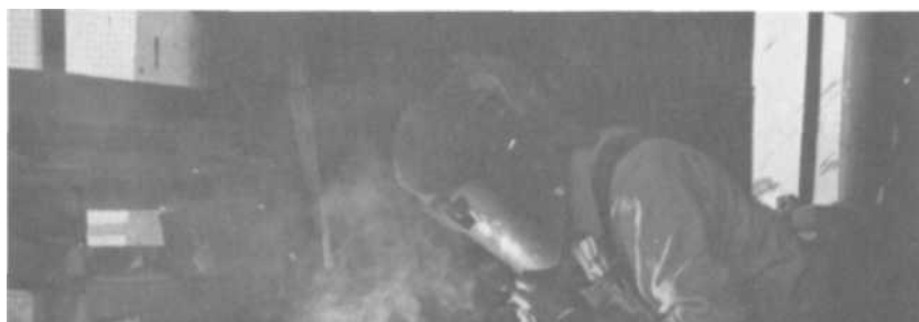
PLATE 80 The steel stock for the band is chosen, measured, bent in a vise, and the ends welded together.
