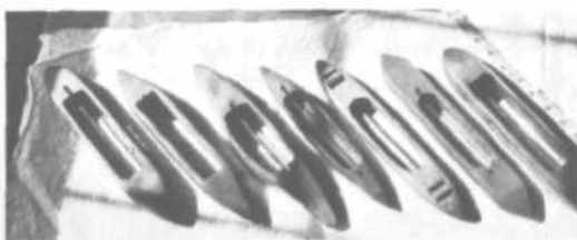
PLATE 251 SHUTTLES come in many different styles and sizes. Their function is the same, however—to carry the thread across the warp, thus creating the weft.
