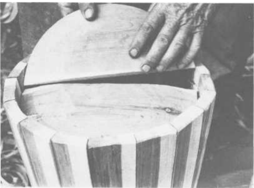
PLATE 366 Step 13: Take the bottom (head) hoop off. Fit the two halves of the head into the groove made by the croze. Put another temporary hoop on that fits in the middle of the churn. (Alex replaced the bottom wooden hoop with a metal middle hoop.)
