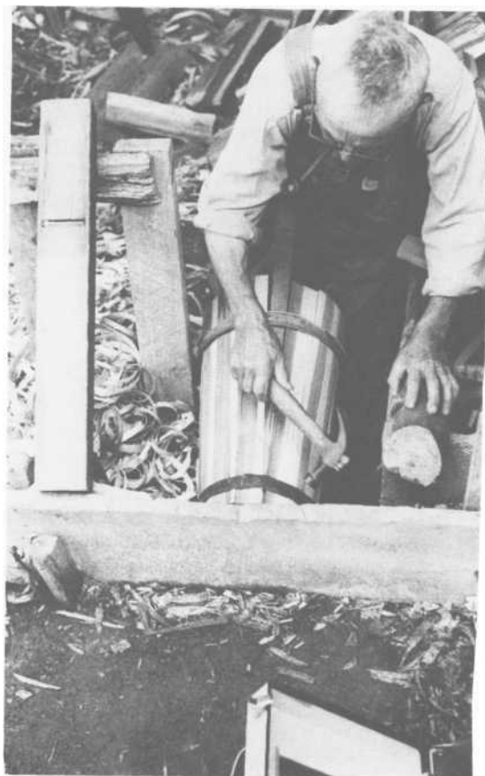
PLATE 347 Step 5: Use a hammer to fit in the last stave. If it won't fit, adjust the other staves with the jointer. A tight fit is absolutely necessary.
