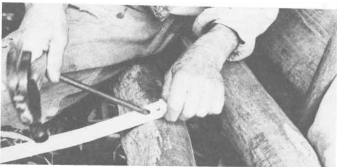
PLATE 377 Make a second hole with the chisel.
