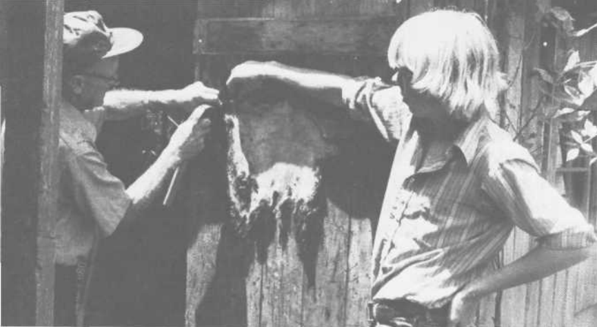
PLATE 22 In its place is tacked the soaking-wet groundhog hide. It will be left there until completely dry and stiff, and then stored for use. Just before use, he will cut out the head, soak it in water to make it pliable again, and tack it onto the banjo while still moist. As it dries, it will tighten on the instrument.
