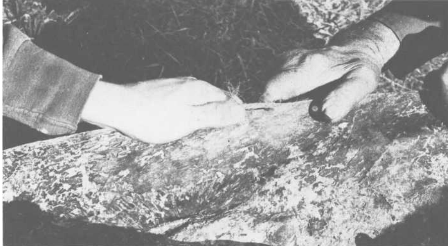
PLATE 32 After the lace is sliced off, he drives a nail in a post and draws it rapidly back and forth against the nail to remove the hair. For longer strips, he cuts in a circle and joins two strips together as described in this chapter.
