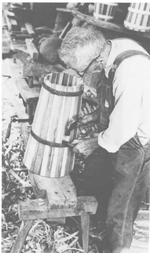
PLATE 367 With a chisel and hammer, force the middle hoop down as tightly as possible.
