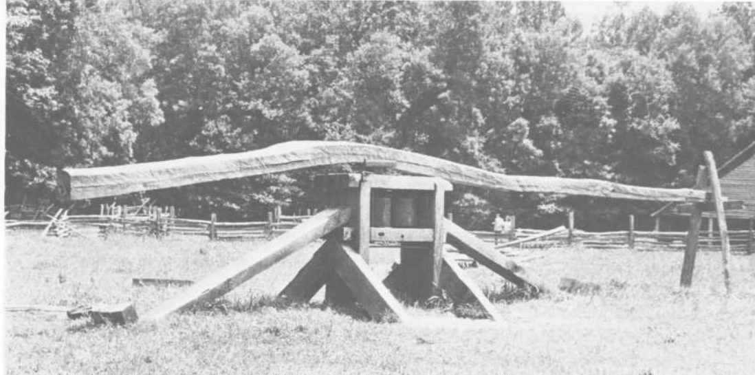
PLATE 411 A horse-operated sorghum mill in the reconstructed pioneer settlement at the Cherokee, North Carolina, entrance to the Smokies.
