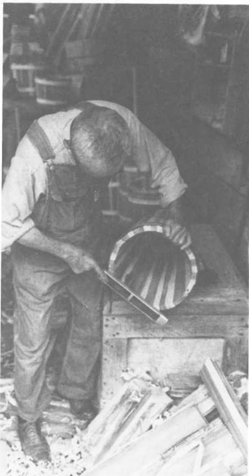
PLATE 352 Step 8: Use a rasp to smooth the outer edges of the top and bottom. The churn must sit straight and flat.
