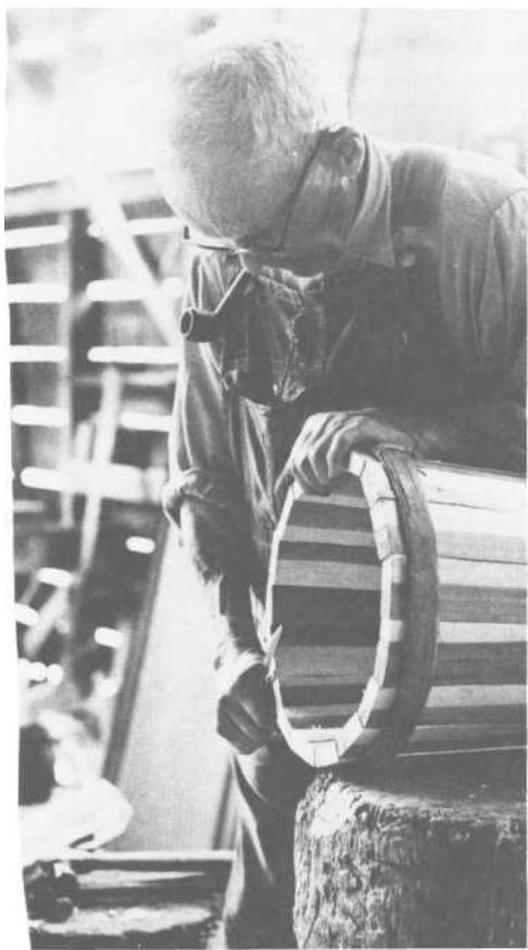
PLATE 349 Step 6: Pull out the bag and hammer the staves until they are even.
