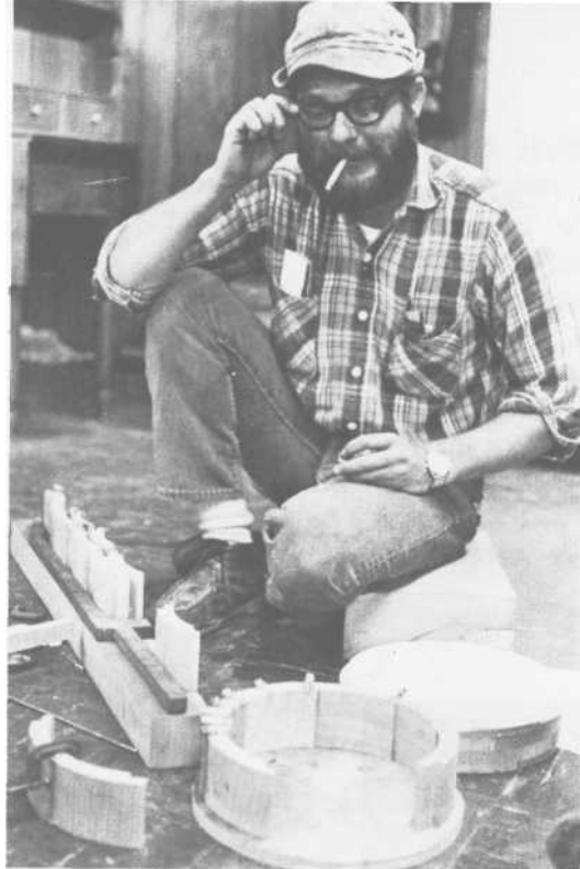
PLATE 127 Dave has his pieces figured out so carefully that he can get every wooden piece he needs out of one 4o"X3"X3" piece of stock.
