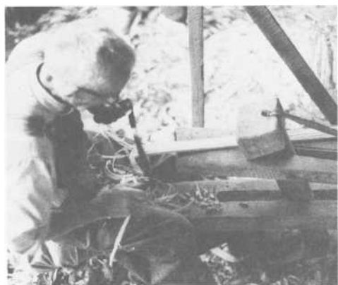
PLATE 373 Step 17: With a drawing knife and shaving horse, smooth the oak pieces to \frac{1}{8} to \frac{1}{4} inch thick and 1 to 1\frac{1}{4} inches wide.
