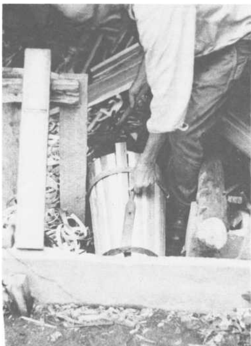
PLATE 348 A chisel can be used as shown to help fit the last stave.
