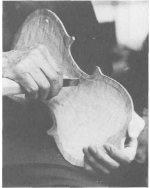
PLATE 129 Garrett shapes the inside concave surfaces and the outside convex surfaces of the top and back with his chisels.
