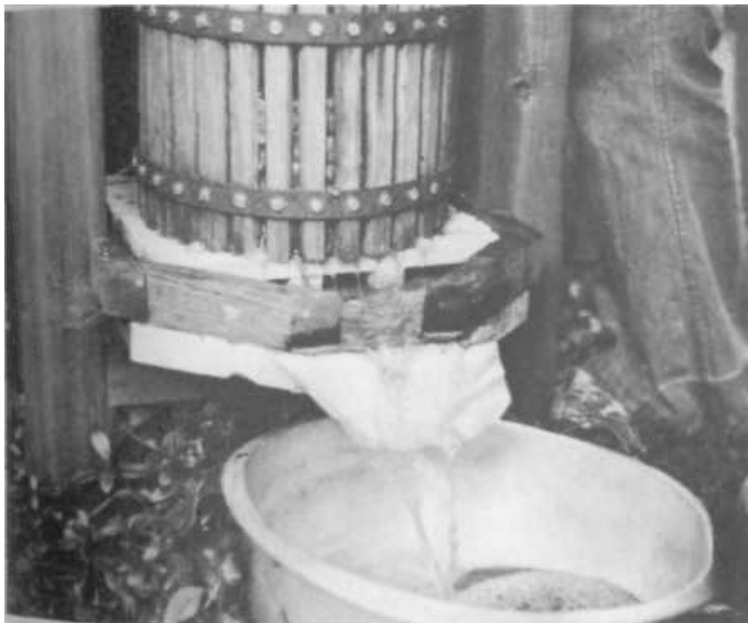
PLATE 396 Tommy Lamb, using a board for extra leverage, turns the handle of the screw to press the juice out. Matt Young and Jim Renfro begin to fill a second tub with pulp.
