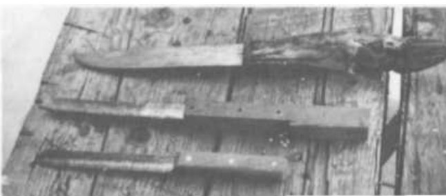
PLATE 25 The knife at the top has a handle made from a deer's foot. The other three knives show various stages of construction of the knife we just saw Tedra make.
