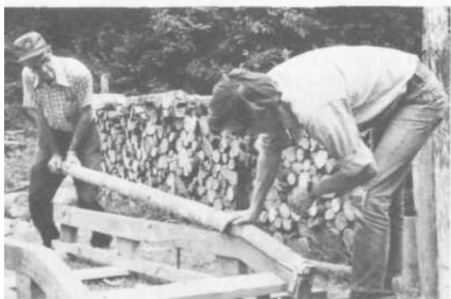
PLATES 176-177 Tedra nails a metal strip to the front of each runner, then he fits the front end of the half sole into it and bends it over to fit the runner's curve.
