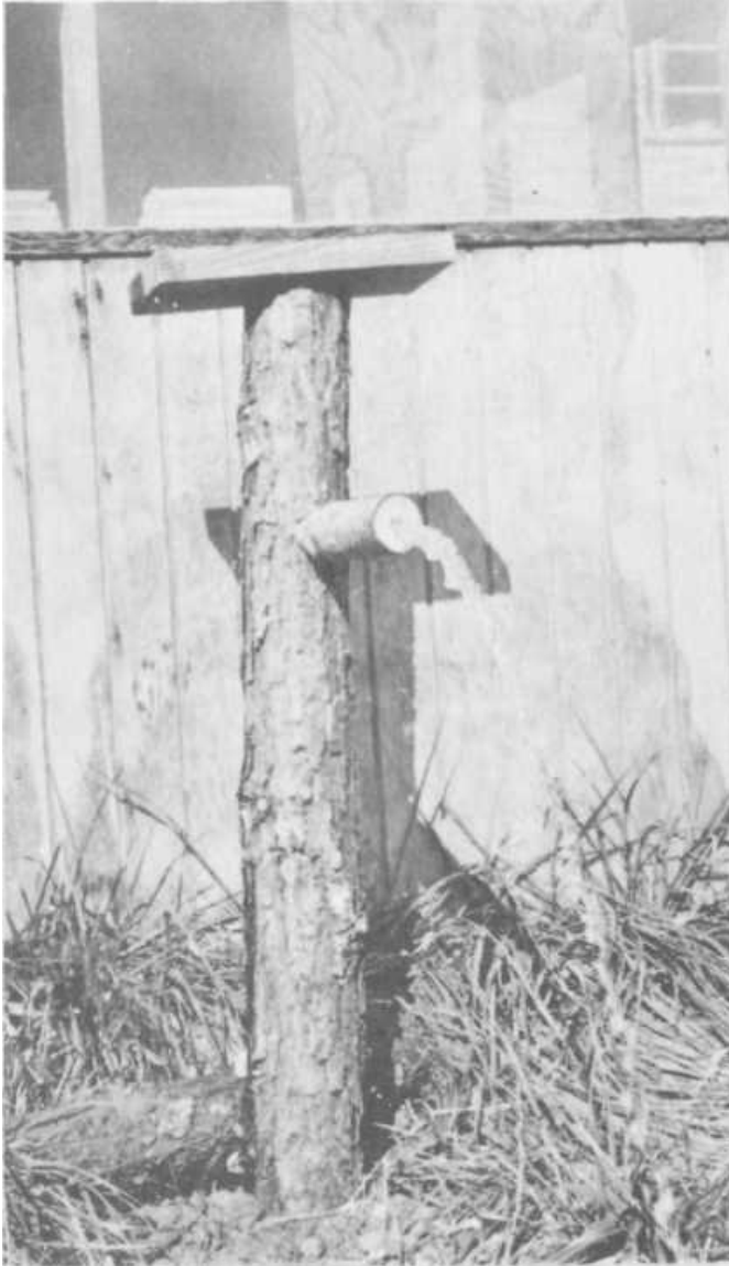
PLATE 315 The finished spigot. The plank on top is nailed firmly in place to prevent the water from shooting out the top through the bored hole instead of the poplar spout in the side.
