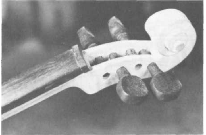
PLATE 117 The neck of the fiddle has been cut out of a block of maple 9"X2 1/4"X2 1/4". It is shaped with a pocketknife and sandpaper. The end may have any design you want. Pegs are tapered so they will tighten in their holes.
