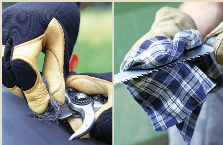
(left) Use wire wool to remove any dried sap from secateurs, and to keep the blades from sticking together. (right) Rub lubricating oil on your pruning saw to protect the blade.
