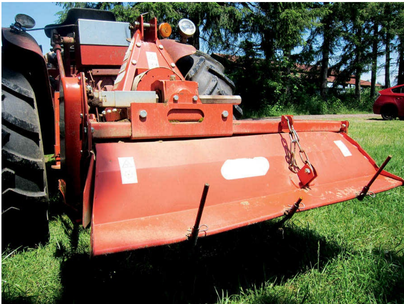
ABOVE: Danny's offset rototiller on the back of his tractor with the rebar row markers
