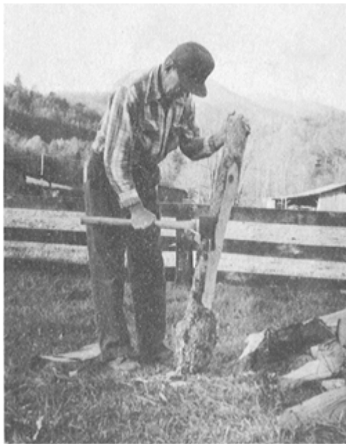
PLATE 461 Carlton shapes the handle by hewing off the excess wood. There was a slight curve in the trunk, so Carlton hewed more off one side than the other so he'd have a straight handle.
