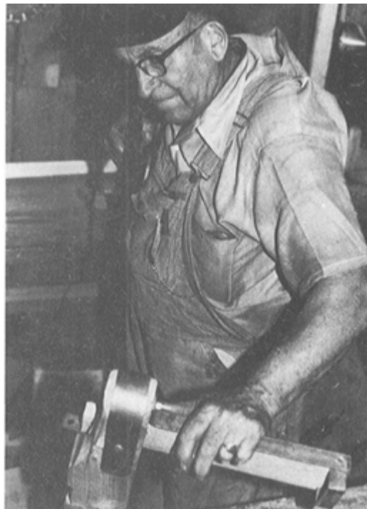
PLATE 316 ... saws any excess off the tenon ...
