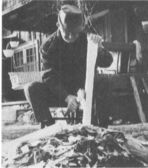
PLATE 468 As the handle approaches the right dimensions, Frank leaves the end that fits into the axhead larger, as well as the opposite end. He continues shaping, taking small, careful cuts. "I make that knot in the end so you can hold it there."
