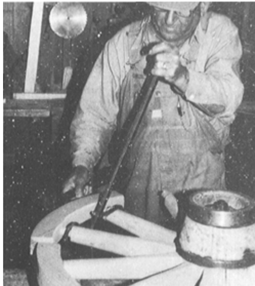
PLATE 240 Placing the felloes on top of the spoke tenons and using a framing square, he marks the location of the holes he will need to drill for the tenons, drills these holes through the felloes from the inside, and then, drawing the spokes closer together with a spoke puller of his own design so that the tenons will hit the holes on the inside of the felloes, he drives the felloes on. As each felloe is driven on, the spokes spread back apart to their original spacing.
