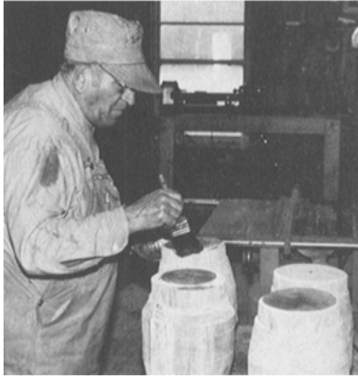
PLATE 200 When all four hubs have been shaped, Jud paints melted paraffin wax on the ends to try to prevent checking (splitting) since the wood for these hubs had only seasoned for a year.
