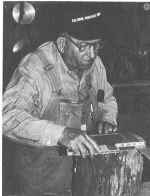
PLATE 189 Now Jud removes as much of the excess wood as he can before mounting the hub in the lathe for the final turning. Here, he prepares to square the block to ten and one-
