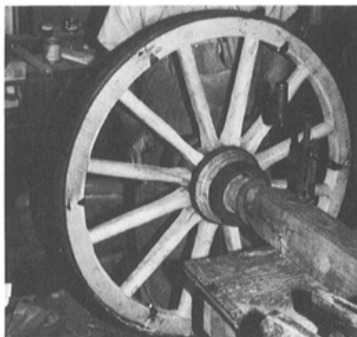
PLATE 284 Then he clamps the axle to his workbench ...
