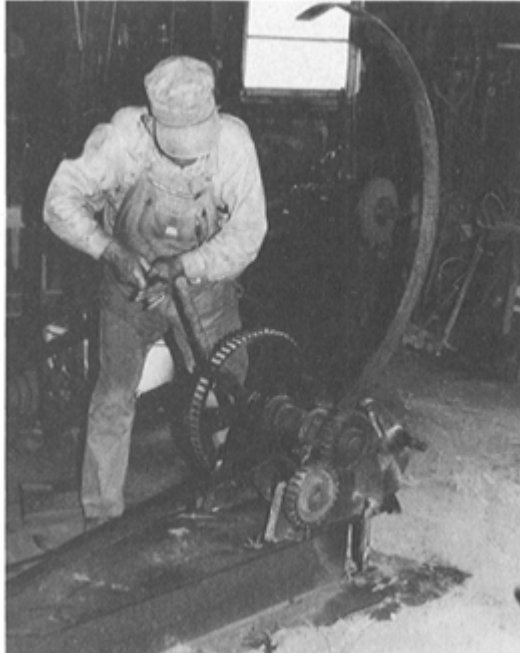
PLATE 250 After cutting the flat bar to the right length for a tire, Jud feeds it into a tire bender which curves it evenly into a hoop.
