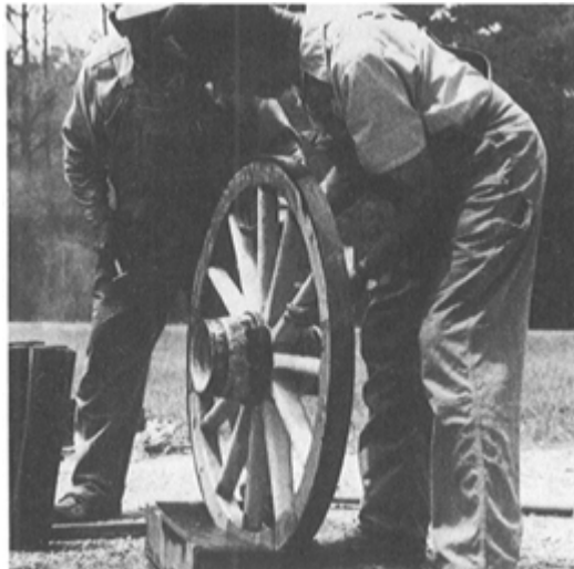
PLATE 264 When the tire is in place, the wheel is immediately taken off the wheel bench and rotated in a trough of water to cool the hot metal and cause it to draw even more tightly against the wheel.
