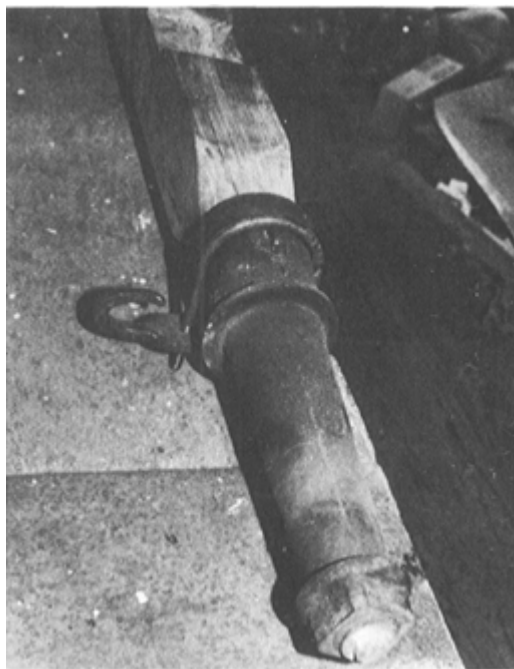
PLATE 306 The plate through which the ends of each thimble U bolt pass is shaped into a hook in front to which the slay chains will be hooked when the wagon is in use. The threads for each thimble's nut are made to keep the nut from unscrewing while the wheel is rotating.
