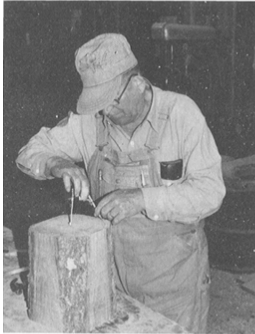
PLATE 194 With a nail set, he punches a shallow indentation into the center of each hub, and then draws a circle eight and one-half inches in diameter on each end with a compass.
