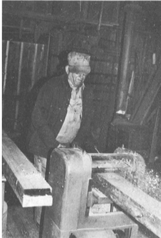
PLATE 295 The sand board is planed, cut out, and then shaped with a drawknife ...
