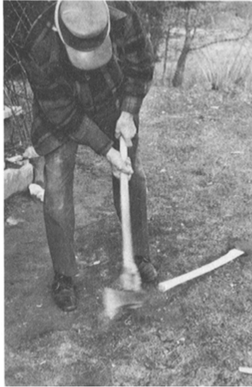
PLATE 476 Now he puts the handle into the axhead. He does this by getting the handle started into the hole and then striking the opposite end sharply six or eight times with a go-devil.
