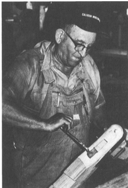
PLATE 317 ... and bends the other end of the metal band that wraps the stake over ...
