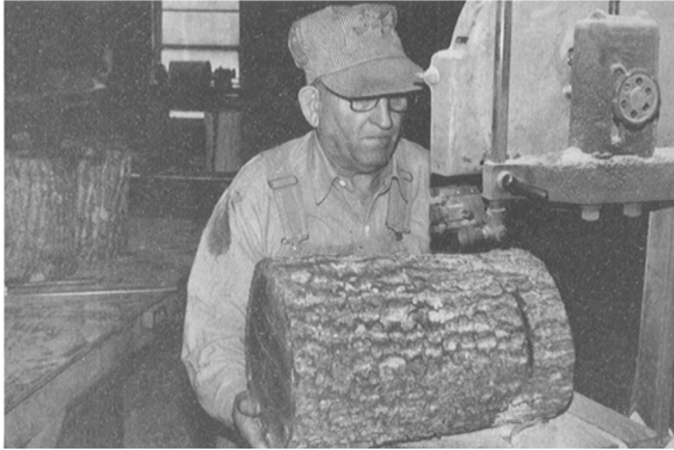
PLATE 188 Using a band saw, he cuts each piece to approximately fourteen inches in length, longer than the final hubs will be, but Jud says, "I just trim 'em off a little long. Got to cut 'em again anyway." Then he removes the bark with a drawknife.
