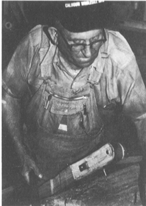
PLATE 317 ... and bends the other end of the metal band that wraps the stake over ...
