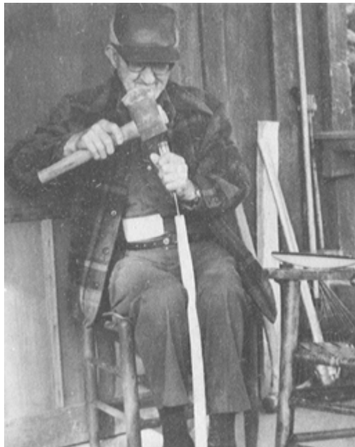
PLATE 473 When he is confident the handle will fit into the head, he takes his chisel and splits the head end open to a depth of four inches.
