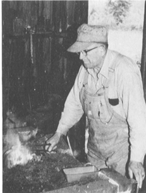
PLATE 214 The bands finished, Jud heats one of the outside bands to approximately 900 degrees Fahrenheit on a black heat.
