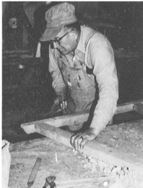
PLATE 291 The crossarm for the front hounds is mortised, and fitted over tenons cut in the hounds' ends.
