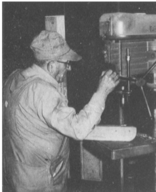
PLATE 290 The necessary holes are drilled for bolts, all of which will be countersunk.
