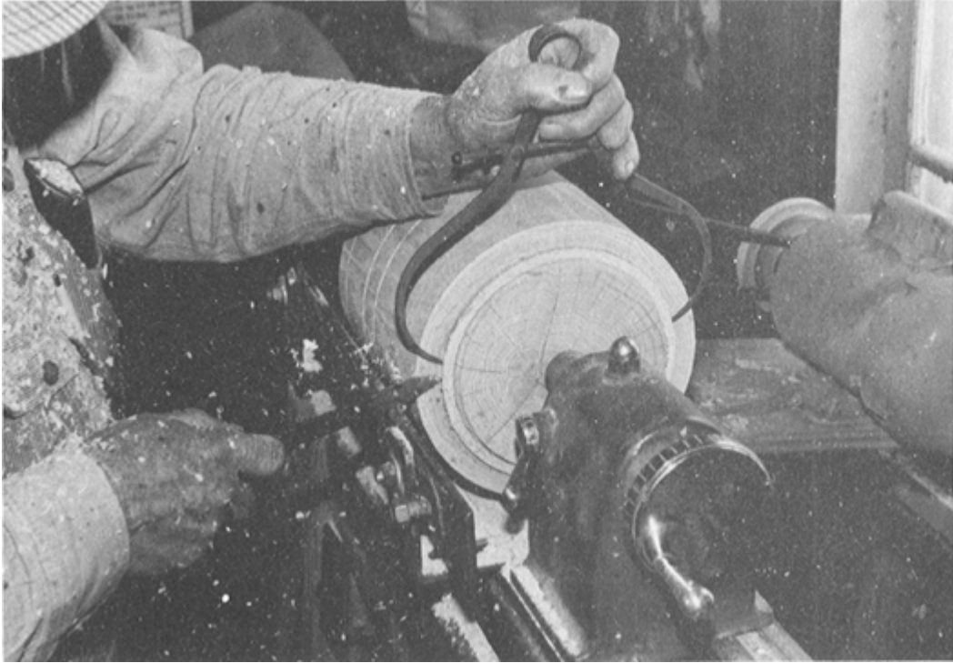
PLATE 198 The end of the hub that will go next to the wagon and hold the bearing is turned to six and one-half inches in diameter. Note that he has also scribed a pair of lines around the belly of the hub. The mortises for the spokes will be fitted in between these lines.
