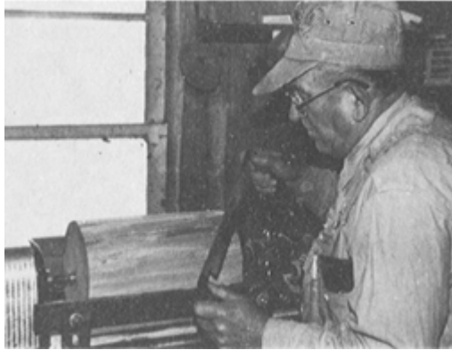
PLATE 196 Now Jud mounts a hub in his lathe, and before starting to turn it, he removes some of the remaining corners and rough spots with a drawknife.
