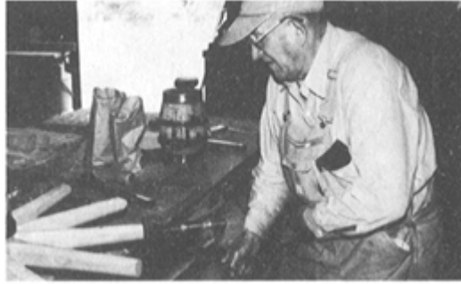
PLATE 233 With the spokes in place, Jud uses a spoke pointer on a brace and bit to shape the ends of the spokes into cones (note the end of the spoke immediately behind the pointer).
