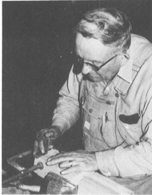
PLATE 311 First Jud cuts out the stakes and mortises out channels for their hardware (made of mild steel, three sixteenths of an inch by three quarters) ...
