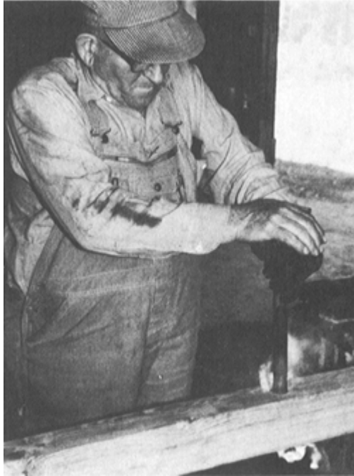
PLATE 299 ... Jud prepares the hole in the center of the bolster for the kingpin, which will allow the front axle and sand board to turn freely under the bolster.
