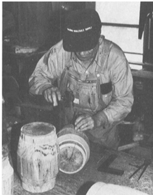
PLATE 201 The two-and-one-quarter-inch mortises for the hub's spokes must now be cut. He subdivides the space between the scribed lines into twelve equal parts for the front hubs and fourteen for the rear, using a small traveler to get the circumference and dividers to establish the dividing lines. With a center punch, he makes three small holes on each dividing line to guide the drill he will use to cut out the mortises.
