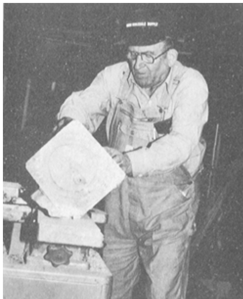
PLATE 195 With the diameter established, Jud now can remove additional excess wood from the corners at a forty-five-degree angle with his joiner. It would be extremely difficult to turn on the lathe with the corners left on.
