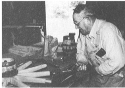
PLATE 234 With the cone as a guide for the hollow auger or spoke auger, he can now shape the ends of the spokes into the round tenons that will go into the felloes (fellies). (Since the felloe end of the spoke is the weak end, the trick is to have as large a tenon as possible to hold the felloes on without breaking off, and yet small enough to leave a good bearing surface for the felloes. According to Practical Carriage Building , many makers leave half the width of the tenon—a fourth on each side—for shoulders.
