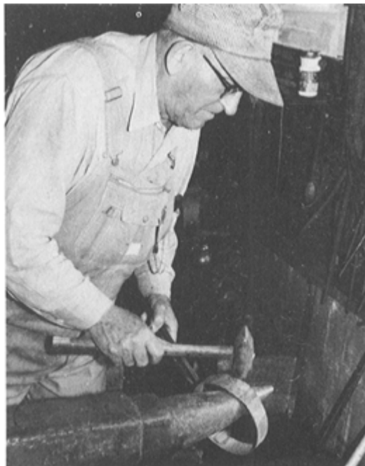
PLATE 213 As each weld is completed, Jud dresses up and rounds each band at the weld's seam before taking it to the cone mandrel.
