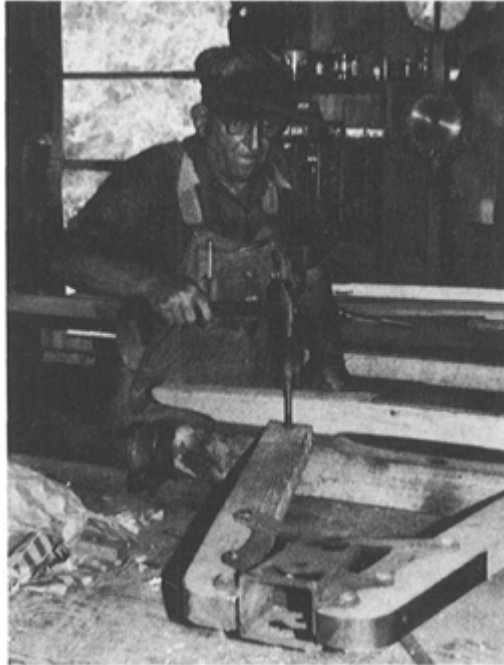
PLATE 307 Now U bolts are made (note that these are flattened in the curve) and holes drilled in the hounds to pin the hounds, sand board, and front axle together.
