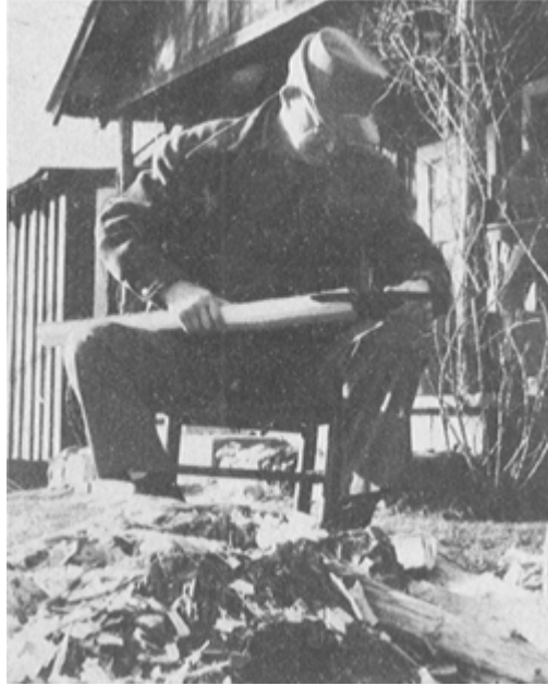
PLATE 466 Once Frank has the piece of hickory chopped down into a rough rectangular slab, he rounds off the corners with his hatchet, and then he holds the axhead against one end to gauge his progress.
