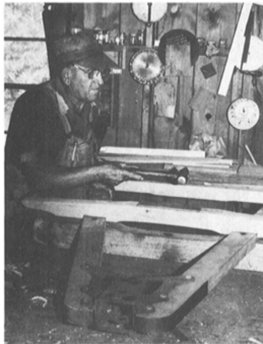
PLATE 298 Placing the front axle, hounds and sand board together ...
