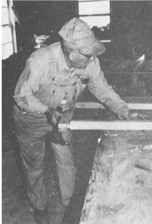
PLATE 291 The crossarm for the front hounds is mortised, and fitted over tenons cut in the hounds' ends.
