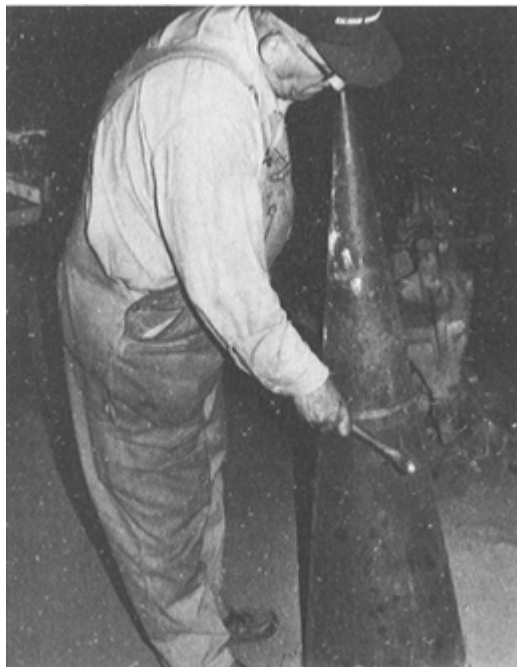
PLATE 211 ... and then driven over a cone mandrel to true them up and make them perfectly round.
