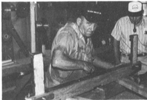
PLATE 325 ... and cuts the mortises in its underside for the hounds and the coupling pole or "reach." The reach will connect the front and rear assemblies, and holes will be drilled in it at intervals for a metal pin which, when pulled, will allow the front and rear axles to be either pushed farther apart or brought closer together as the wheelbase needs to be changed to accommodate the job at hand.
