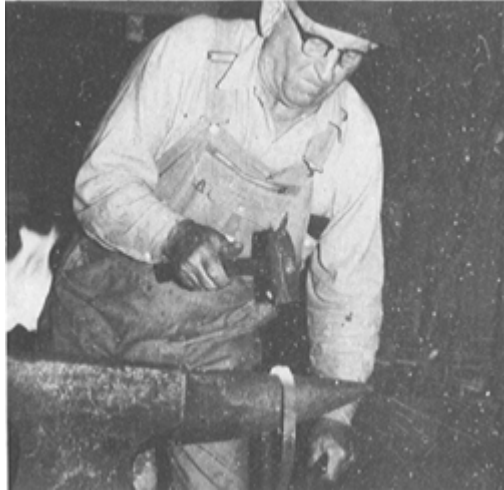
PLATE 210 The ends of the inner hub bands are now forge-welded together ...
