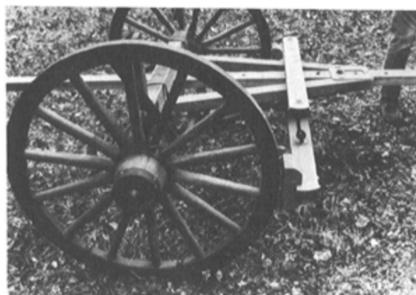
PLATE 330 Now the wheels are added, and the coupling pole, and the two halves pinned together.
