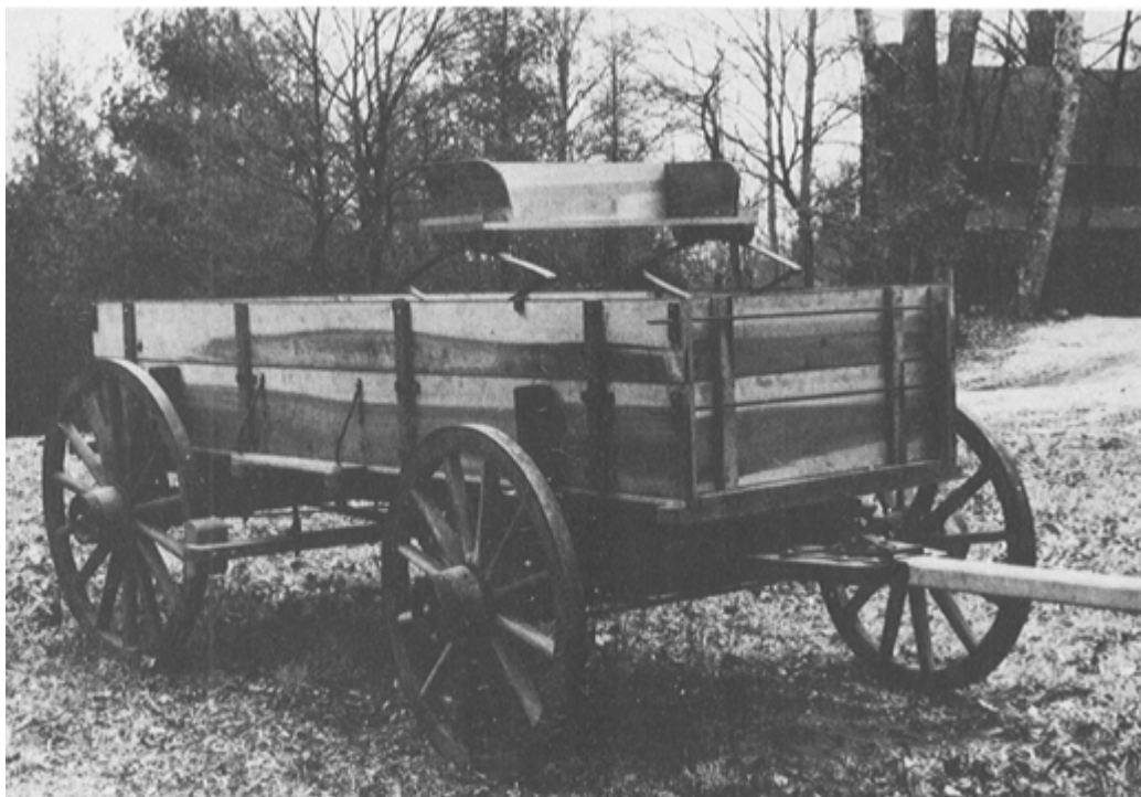
PLATE 335 Last, Jud makes the bed and seat and then places it on the frame between the standards.
