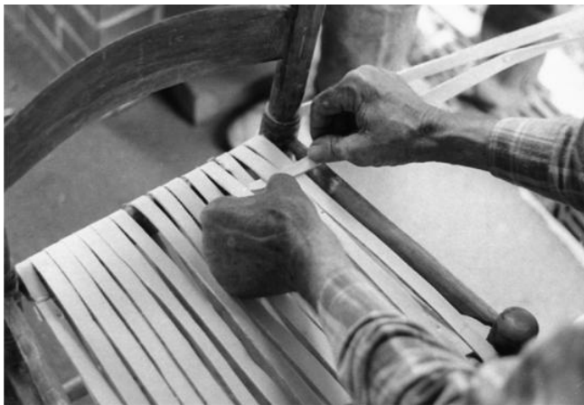
PLATE 166 After completely wrapping the seat in one direction, Nelson started weaving the strips across the chair. The pattern he chose was a simple under-over pattern. Although the weave felt loose at first, it began to tighten as more rows were woven.
