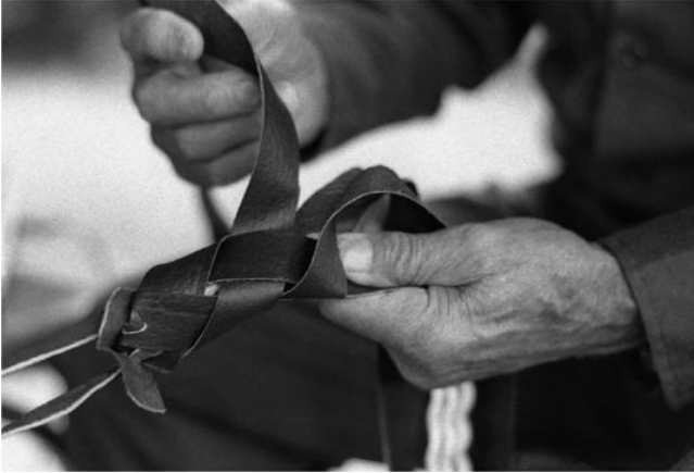
PLATE 190 He begins the braiding of the bullwhip, braiding the leather tightly around several strands of cotton rope. (He prefers a thick piece of rope to give more bulk to the upper section of the whip but used a piece of unraveled clothesline in this demonstration. The rope is doubled and pulled through the leather loop so that it will not pull out as the whip is braided. Note one of the loop's ends protruding from the top of the braiding to show how it has been worked into the whip.)
