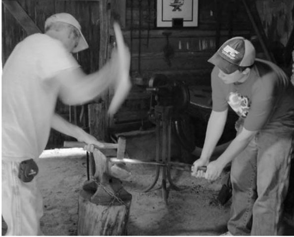
PLATE 176 Ben holds the hot metal with tongs as Barry strikes the hot-cut chisel with the hammer
