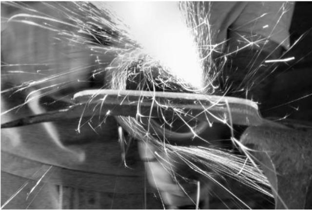
PLATE 179 The cutting edge of the drawknife being ground with an angle grinder. The back of the blade is being lightly touched up after heavier grinding on the front.
