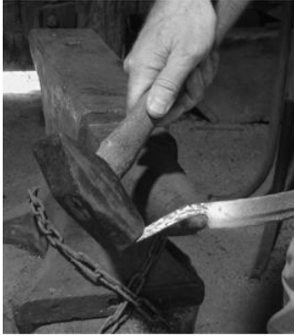
PLATE 180 A tang is hammered down while being held against the point of the anvil horn.
