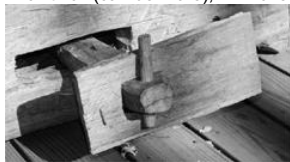
PLATE 153 The foot pedal is held on the dumbhead shaft by a peg.
