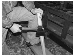
PLATE 145 Rough shaping of the legs with a hatchet
