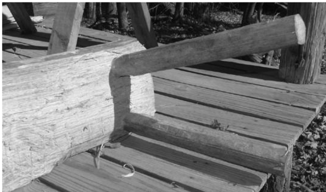
PLATE 148 The bench (on its side) with legs inserted
