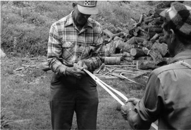
PLATE 160 When they got to Mrs. Echols's house, they peeled off the outer bark, leaving the white, pliable inner bark, which was used to bottom the chair. Nelson, left, and Elvin, right, splitting a piece of inner bark (that they've already scraped the rough outer bark off) into two pieces, about \frac{3}{4} to 1 inch wide
