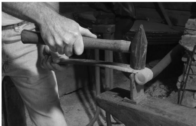
PLATE 175 The end of the leaf spring being cut off on the hot-cut hardie
