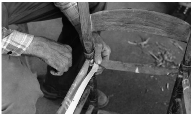
PLATE 162 To begin bottoming the chair, a strip is folded over the chair round at the back of the chair. To hold the strip in place, tiny notches were made on either side of the strip, above and below the round, and then tied with a piece of string, looping it over and over about ten times.
