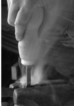
PLATE 181 A wooden handle being pushed into a heated tang, creating smoke
