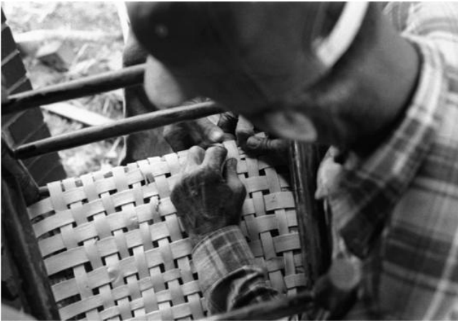
PLATE 168 To complete the chair bottom, the end of the last strip is woven back through the last two or three vertical rows, leaving no loose ends.
