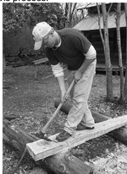
PLATE 143 Shaping the bench with an adze
