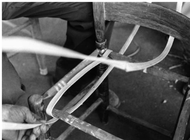
PLATES 163 AND 164 This strip was about 20 feet long. We began looping it around the front and back rounds as shown in these two pictures.
