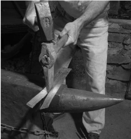
PLATE 177 The piece of leaf spring being cut lengthwise using the hot-cut chisel
