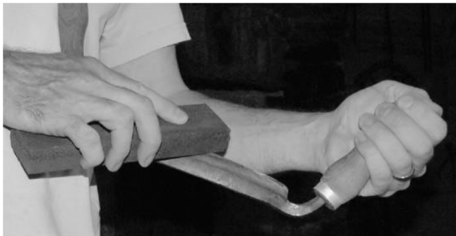
PLATE 182 Sharpening the finished drawknife with the whetstone
