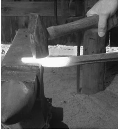
PLATE 178 A shoulder and tang being formed by hammering down with the hammer face half over the anvil and half off it
