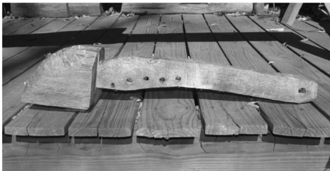
PLATE 149 The dumbhead with all mounting holes drilled: foot-pedal hole at the bottom (right), mounting holes just below the head
