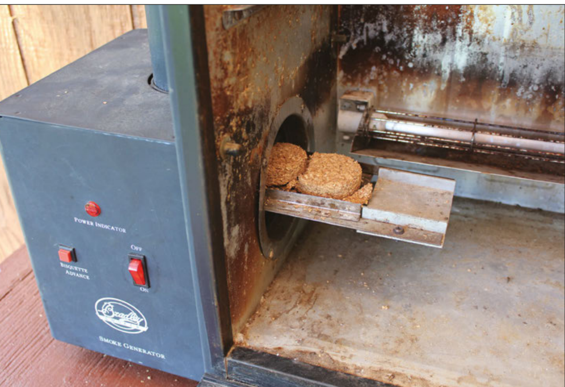
ABOVE: The smoke generator feeds bisquettes at a precise burn time of 20 minutes per bisquette.
